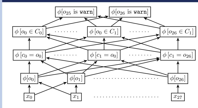
Partial example of an event **network** with five layers encoding, highly interconnected events for clusters  $C_0$  and  $C_1$ .
