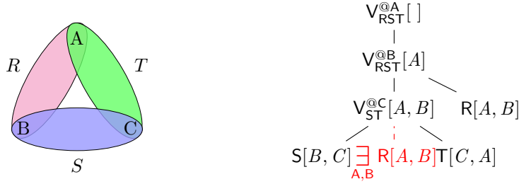
Figure 6: (left) Hypergraph of the triangle query Q_{\Delta} ; (right) View tree for the variable order A - B - C with an indicator projection \Xi_{A,B}R .
