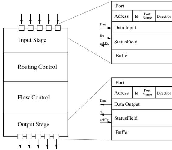
**Fig. 3.** A router and its ports
