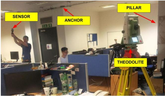
Figure 2. An electronic theodolite is used to obtain a millimeter-resolution ground truth. Four anchors are placed on roof runners, and a single tag sensor is carried around the room. The sensors records inertial, geomagnetic, time-of-flight and received signal strength measurements for processing offline.
