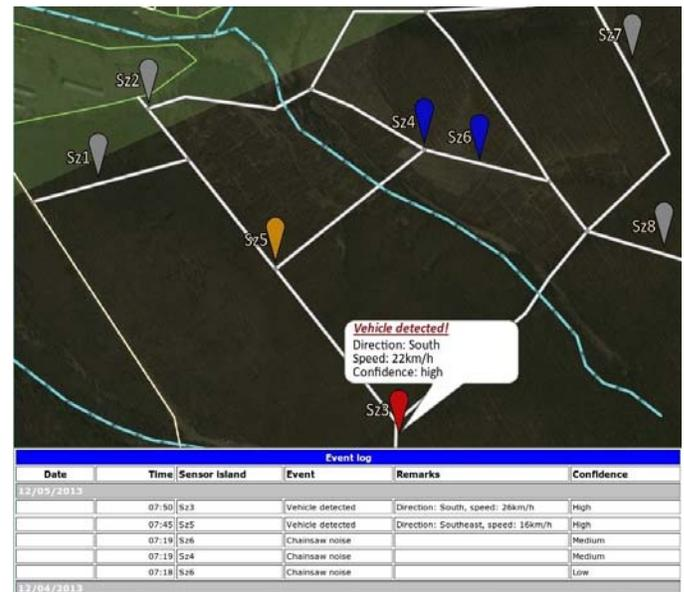
Fig. 3. Prototype monitoring screen of the surveillance system. Sensor islands are represented by colored bubbles. Detected events are listed below the map.
