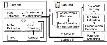
Fig. 5. The architecture of the proposed system, where the front-end runs on the user carried devices, and the back-end resides on the cloud.
