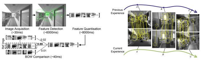
Fig. 2. Typical processing pipeline and running time (estimated on a Google Glass) of the Bag-of-Words image comparison approach [9].
