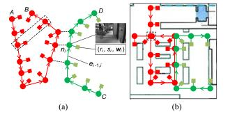
Fig. 4. (a) Two annotated experiences, where each node  $n_i$  is associated with visual processing parameters  $(r_i, s_i, w_i)$ . The dashed lines are co-location links, through which the user can transit from one experience to another. (b) The global embedding of the annotated experience graph over the floorplan.
