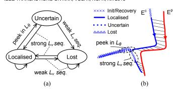
Fig. 12. (a) The decision model used by our system to handle localisation failure. (b) An example where the user tries to explore a new route.
