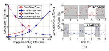
Fig. 16. (a) Localisation accuracy and energy consumption under different image sampling intervals. (b) Normalised CPU load of NaviGlass (top) and L-Learning (bottom) when sampling images every 4s.
