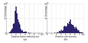
Fig. 18. Distance travelled between (a) the actual deviation point and when detecting localisation failure, and (b) the actual return point and when successful localisation is resumed.
