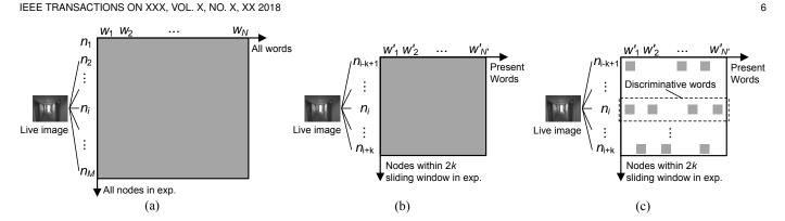
Fig. 8. During localisation, a live image can be compared with (a) all nodes using the complete vosual vocabulary (standard approach); (b) a sliding window of nodes using only the present words (after parameter initialisation); and (c) the most discriminative words (after parameter learning).
