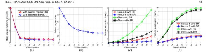
Fig. 19. (a) Mean image matching error at different image scales, with/without salient region detection. (b) Relative sizes of the detected salient regions (percentage comparing to the full image) at different scales. (c) Running time of feature detection, and (d) quantisation at different image scales.
