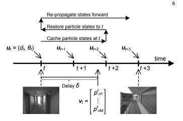
Fig. 11. The proposed system handles the delayed visual measurements by rolling back to particle states when the images were taken, and re-propagating the states with the user motion observed afterwards.
