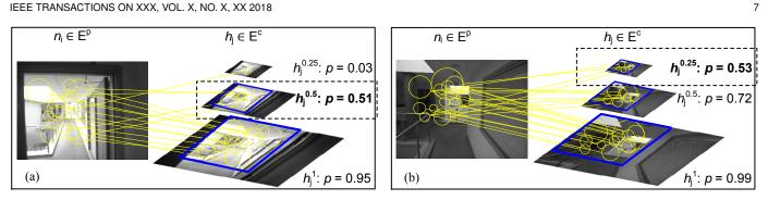
Fig. 9. Matching results of image pyramids for cases where dominating features are (a) far away from; and (b) close to the camera. Blue bounding boxes illustrate the estimated salient regions at different layers.
