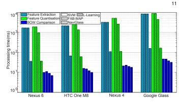
Fig. 15. The running time of feature detection and quantisation per image for different devices. The proposed approach is up to  $50 \times$  faster than the competing algorithms.
