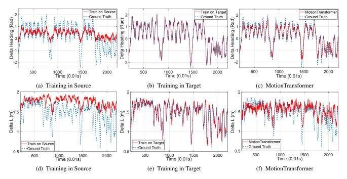
Figure 3: Heading displacement estimation from training in (a) source domain, (b) target domain and (c) MotionTransformer, and location displacement estimation from training in (d) source domain, (e) target domain and (f) MotionTransformer
