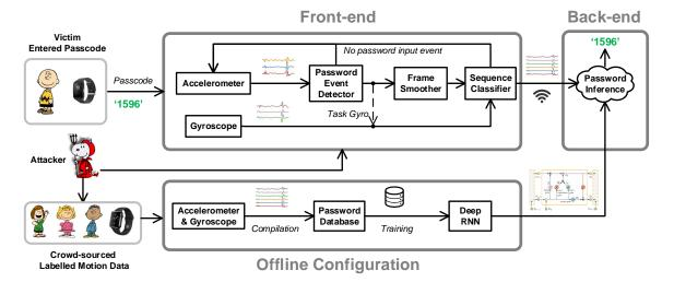
Fig. 3. System overview:The attacker builds a deep RNN classifier using crowd-sourced data. On a victim's smartwatch, a trojan app uses an adaptive sampling scheme to record and identify a victim's motion data. Candidate password sequences are uploaded to the server. The back-end server runs the trained deep RNN classifier to infer possible passwords. Note, training is only required by the attacker; no training is needed by the victim.
