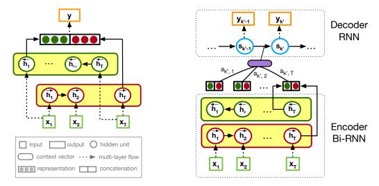
Fig. 5. The architectures of two inference models in Snoopy. Left: seq2pwd Model for commonly used password inference. Right: seq2dgt model for universal password inference.
