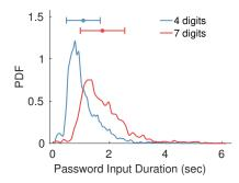
Fig. 6. PDF of APL input duration. Left: duration distribution of swiping APLs. Right: Differentiating a 4-digit APL and 7-digit APL is difficult based on their duration distribution.
