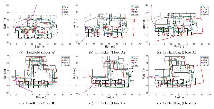
Fig. 7: Our proposed IONet can generate more accurate trajectories in large-scale localization experiments on two office floors - Floor A (1650  $m^2$ ) and Floor B (2475  $m^2$ ) in three attachments - Handheld, In Pocket, and In Handbag, compared with SINS and PDR. Note that our learning model is trained inside one room (Vicon Room), but generalize well to outside places without further training.
