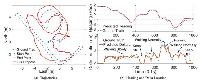
Fig. 8: The performance of IONet is evaluated on an challenging experiment with varying motion modes including waking slowly, halting, walking normally and running for estimating (a) trajectory and (b) heading and location displacement. IONet can learn an extensive amount of information about the idiosyncratic motion behavior associated with different motion modes.
