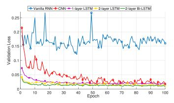
Fig. 4: The losses of adopting various frameworks demonstrate that our proposed IONet framework with 2-layer Bi-LSTM descends more steeply, and stays lower and more smoothly during the training than all other neural networks.
