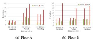
Fig. 10: In large-scale indoor localization, absolute position errors of IONet is calculated at a distance of 50m, 100m and the end point on Floor A (a) and Floor B (b), showing competitive performance over traditional PDR.
