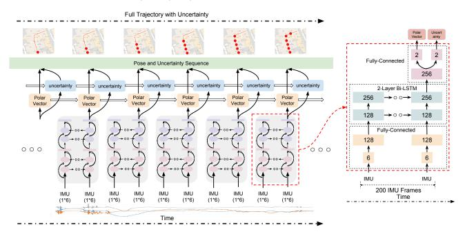
Fig. 3: Overview of IONet framework. Inertial measurements are segmented into independent windows. A 2-layer bi-LSTM is used to estimate the change in heading and displacement (polar vector) as well as the estimation uncertainties.
