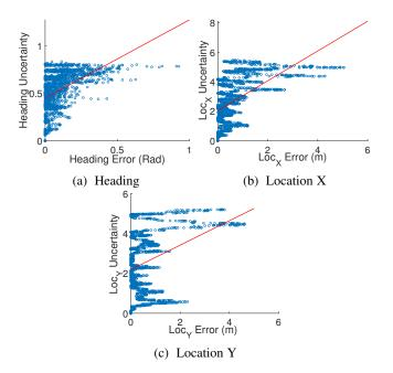
Fig. 12: The correlation between uncertainties and errors for global heading (a) and locations (b, c) demonstrates that the uncertainties are in positive correlation with the errors. Note that the small error does not always mean small uncertainty, because the mean errors can cancel with each other.
