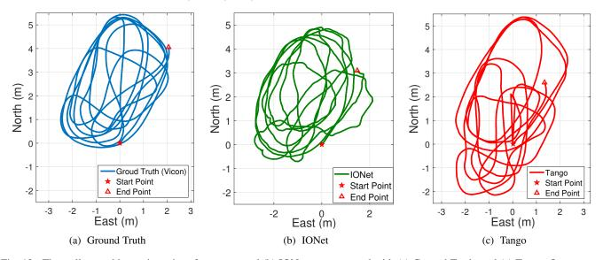
Fig. 13: The trolley tracking trajectories of our proposed (b) IONet are compared with (a) Ground Truth, and (c) Tango. Our proposed IONet shows almost the same accuracy as Tango, and even better robustness, because our pure inertial solution suffers less from environmental factors.
