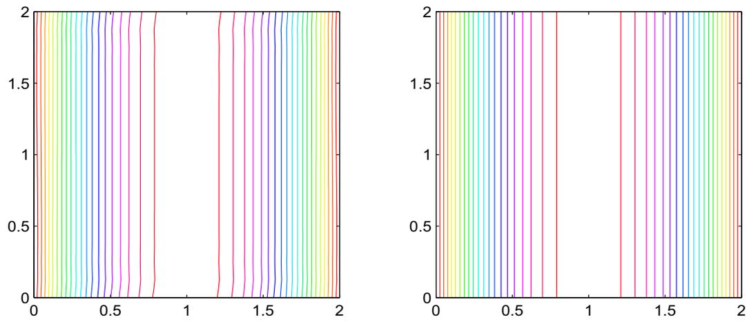
Figure 3: Pressure contours, for  $\sigma = 1$ ,  $\nu = 1$  (left), and  $\nu = 10^{-4}$  (right).
