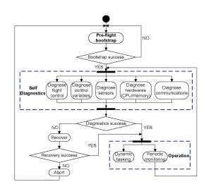
Figure 5: Activity diagram for the phases of operation
