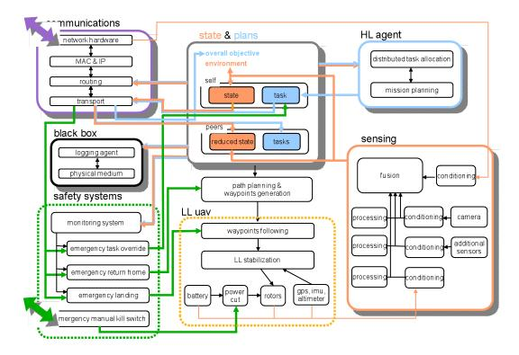
Figure 2: Overall System Architecture
