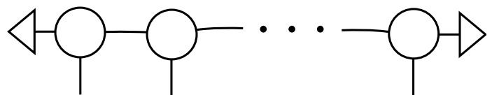
Figure 1: Tensor network states in the current formalism have this generic form. The legs on the bottom index spin degrees of freedom.
