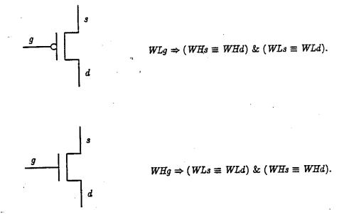
The precondition for connection of a wire to High or Low is that it is not also connected to the other.
