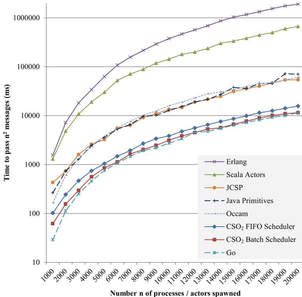
**Figure 4.** Benchmarking the performance of our CSO<sub>2</sub> library, using both the FIFO and batch scheduler, against several alternatives for speed of message passing. Time is the mean wall time in milliseconds for fifty runs on a logarithmic scale (lower is better).
