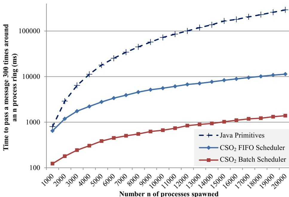
**Figure 5.** Benchmarking the performance of the batch scheduler against both the FIFO scheduler and Java primitives. Time is the mean wall time in milliseconds for fifty runs on a logarithmic scale (lower is better).
