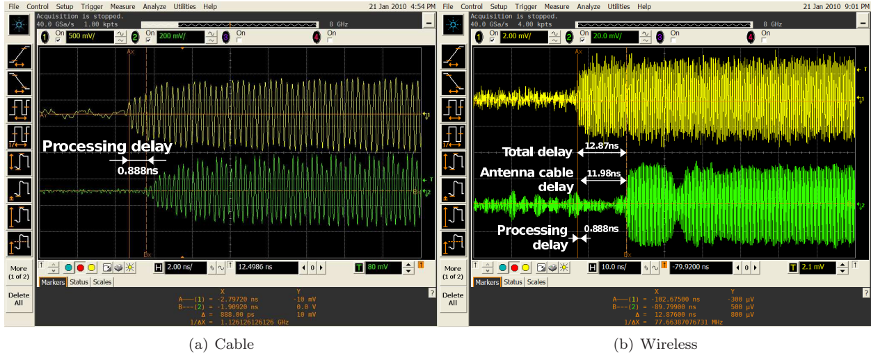
Figure 7: The delay of the prover’s distance bounding radio extension. The top signal is measured at the reception antenna of the provers radio and is transmitted on channel C_0 at 3.5GHz. The bottom signal is measured at the transmission antenna and is being transmitted at the C_2 channel at 4.0GHz. The delay between them, and thus the prover’s processing time is 0.888ns .
