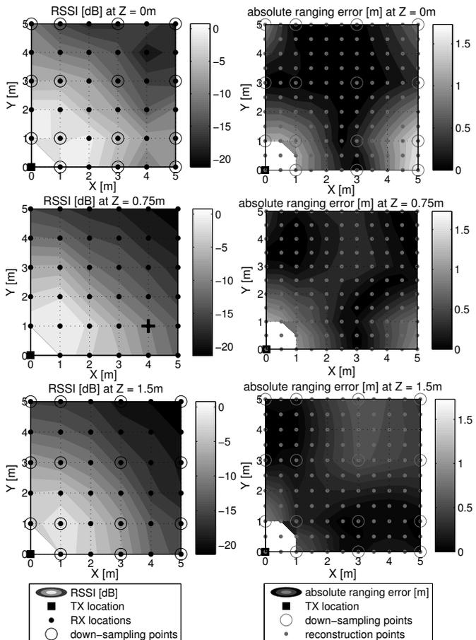
Fig. 1. Sparse magnetic fingerprinting (RSSI – left column) and ranging using the reconstructed RSSI (error in the range estimate  $\hat{r}$  – right column).
