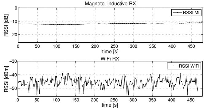
Fig. 3. The RSSI stability over time. Magnetic link vs. WiFi link.
