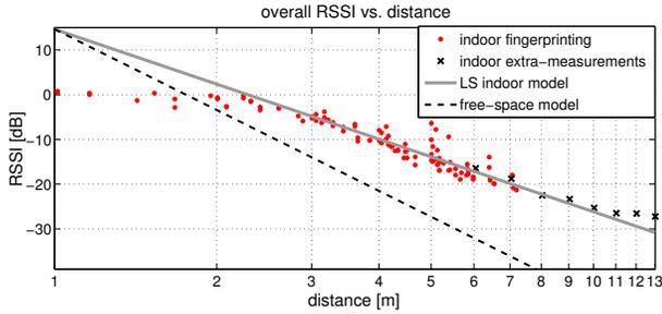
Fig. 2. The decay of RSSI with distance  $r$ . Measurements vs. models.
