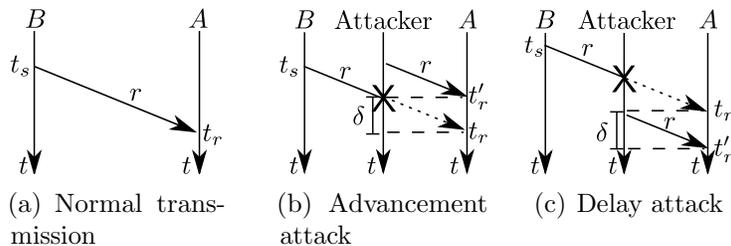
Figure 1: (a) Transmission without an attacker. (b) The attacker sends  $r$  earlier to advanced the message. (c) The attacker jams  $r$  and re-sends it later to delay the message reception.
