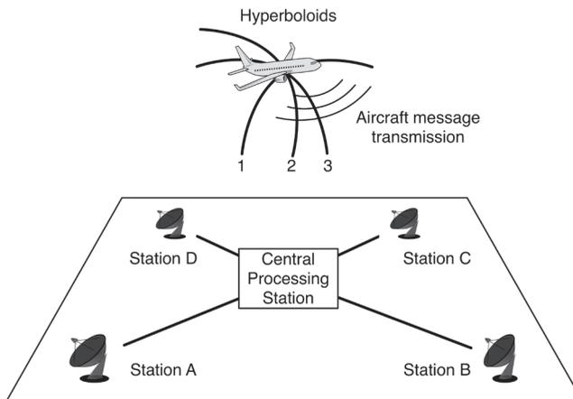
Wide Area Multilateration (WAM) is particularly useful for ATC since it allows location estimation of an aircraft using 1090 MHz messages over large areas. WAM, combined with ADS-B, will form a key part of the next generation surveillance technologies [18] and can help to detect unusual ADS-B reports.
