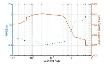
Figure 14: The figure shows the cumulative quality score (CQS) over a period of time as a function of the foreground detector learning rate  $(\alpha)$ . The optimum learning rate according to RMSE maximizes CQS, thus this metric can be used to train the foreground detector.
