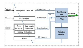
Figure 3: Overview of the proposed system architecture.
