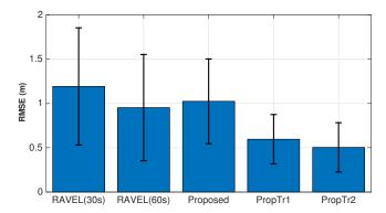
Figure 10: Tracking accuracy between the proposed approach and RAVEL. Proposed denotes our approach where the foreground detector and step-length model are not trained.  $Prop\,Tr1$  is our approach after the foreground detector has been trained and further in  $Prop\,Tr2$  the step-length model is also trained. RAVEL(30s) and RAVEL(60s) is the competing technique evaluated at window sizes of 30 and 60 seconds respectively.
