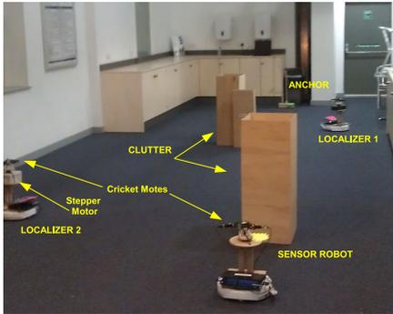
(a) Experimental setup for two localizer configuration. The localizers (with red markers) form a multi-hop distance chain between the sensor robot (yellow marker) and the anchor (in the far end of the picture).
