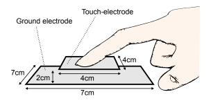
Fig. 6. Signal and ground electrodes are 2 cm apart and manufactured from two aluminum plates.
