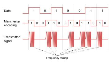
Fig. 7. Data is Manchester encoded. The transmitted signal follows an on-offkeying modulation. During the "on"-periods a frequency sweep is performed.
