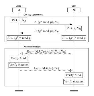
Fig. 4. The pairing protocol uses the wireless channel (solid arrows) for the key agreement and the body channel (dotted arrows) for the key confirmation.
