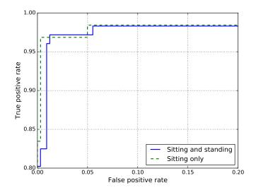
Fig. 10. Receiver operating characteristic (ROC) for the body channel classifier, zoomed into the upper left area. We compare the effect of two body poses: participants are sitting or standing when touching the electrodes (solid line) or sitting only (dashed line).
