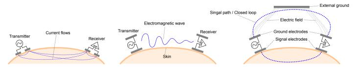
Fig. 1. Three main methods for intra- and on-body channel communication. From left to right: galvanic coupling, surface wave and capacitive coupling.
