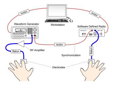
Fig. 5. Measurement setup. A waveform generator transforms the message into an electric signal which is amplified and emitted through the touchelectrode of the transmitter. The touch-electrode of the receiver is connected to a software defined radio which captures the incoming signal.
