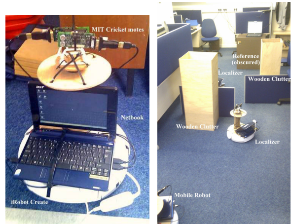
(a) Mobile robot capable of measuring distances using MIT Cricket motes (b) Demonstration of ADAPTPLACDVDIST for two localizers between a reference and a mobile robot/node. Here, the reference is obscured between the wooden clutter.
