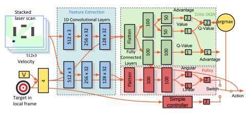
Fig. 2: Network architecture. Network layers are demonstrated by the rectangles. Orange arrows indicate the connectivity between network layers and some other components, e.g. input state and the output of the simple controller. The final action is selected based on the Q value predicted by critic-DQN.
