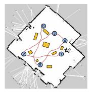
Fig. 11: The trajectory of robot in the real world experiment. The yellow rectangles are obstacles and blue circles indicate the sequential targets.
