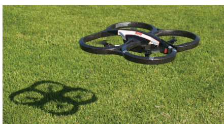
Figure 1: Rotor based UAV with four rotor ‘quad-copter’
