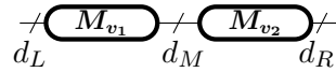
Figure 2.10: Tensor network representing the contraction of a (d_L, d_M) dimensional tensor with a (d_M, d_R) dimensional tensor.
