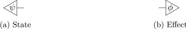
Figure 2.4: Diagram (a) above represents the state |\psi\rangle i.e. a tensor with single output index (a column vector) and diagram (b) the effect \langle\phi| i.e. a tensor with a single input index (a row vector)
