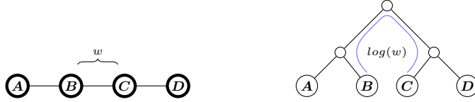
Figure 2.9: Logarithm of bond dimension being routed through the unique path connecting two leaves in contraction tree.
