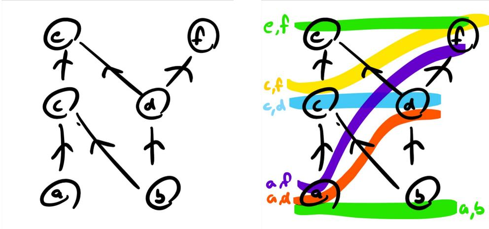
Figure 4.1: Left: the Hasse diagram for a causal order on 6 events  $\{a, b, c, d, e, f\}$ . Right: the maximal slices for the causal order highlighted (all other slices can be obtained as subsets of the maximal slices)[GSC21]
