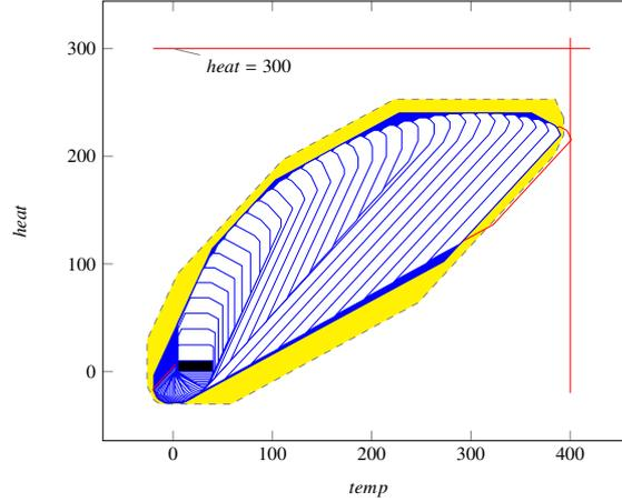
**Fig. 12** The abstractly accelerated tube (yellow, dashed boundary), representing an over-approximation of the thermostat reach tube (dark blue). The set of initial conditions is shown in black, whereas successive reach sets are shown in white. The guards and the reach set that crosses them are close to the boundary in red.
