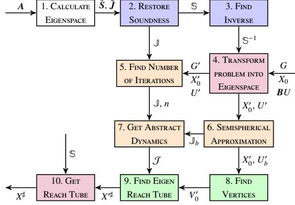
**Fig. 3** Block diagram describing the different steps used to calculate the abstract reach tube of a model via Abstract Acceleration. The white box is the numerical eigensolver stage. Blue boxes are soundness restoration stages. Red boxes represent linear transformations of the problem. The orange boxes denote abstractions defined in this paper, and the green boxes the reachability computation in the abstract domain.
