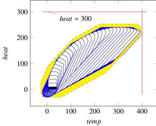
**Fig. 3.** The abstractly accelerated tube (yellow, dashed boundary), representing an over-approximation of the thermostat reach tube (dark blue). The set of initial conditions is shown in black, whereas successive reach sets are shown in white. The guards and the reach set that crosses them are close to the boundary in red.
