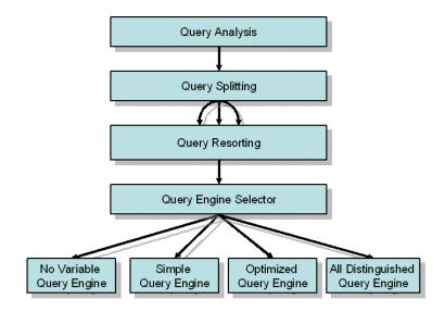
Fig. 4. Components of the query engine
