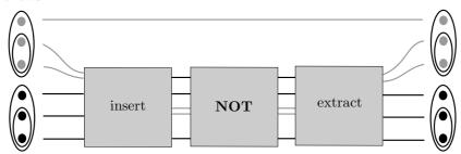
First, instead of inserting 1 anyon, we insert a couple that will be used as a test couple and that in the very same manner as described in a) – as these two will fuse together yielding either 1 or  $\tau$ , this is exactly what we want. Secondly, we apply the  $i\cdot\mathbf{NOT}$ -gate computed in b). Finally, we extract the control pair returning it to its original position by applying the insertion procedure in reverse order. This is done, again, without disturbing the triple at stance here.
