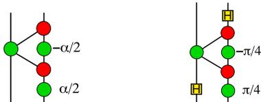
The quantum Fourier transform can be realised as a quantum circuit containing only Hadamard and controlled phase gates; the 2 qubit instantiation of this circuit is shown on the right above. Furthermore, the algorithm can be simulated graphically, as shown in Figure 1.
