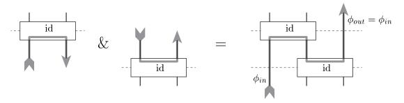
In the above picture neither the one-**eP** input only nor the one-**eP** output only path admits a compositionality statement in the sense of Section 3 but the joint path admits one. Hence one can define the compositional behavior for the output only and the input only path by their behavior within the concatenated path.
