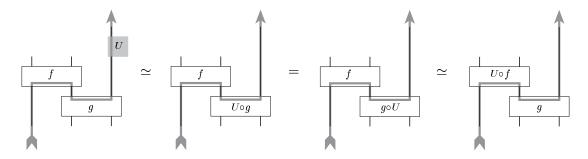
Hence effectuating the unitary action U "at the end of the path" is equivalent to having implemented  $U \circ f$ . Thus we can use U to correct f into the desired result  $U \circ f$ . We now weaken the commutation requirement.
