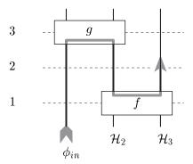
At time 2 the third carrier of state is in general entangled to the second one since they are in the entangled state labeled by an arbitrary function f.
