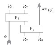
Dually, when we want to implement the composite of functions with matching types e.g.  $f:\mathcal{H}_1\to\mathcal{H}_2$  and  $g:\mathcal{H}_2\to\mathcal{H}_3$ , then the projectors on the states  $\eta^{-1}(f)\in\mathcal{H}_1^*\otimes\mathcal{H}_2$  and  $\eta^{-1}(g)\in\mathcal{H}_2^*\otimes\mathcal{H}_3$  don't match for a "teleportation-style" implementation.
