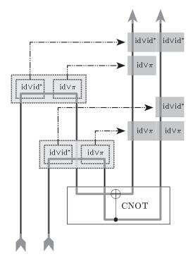
If in this picture we substitute "id $\vee$ id\*" by "Z" and "id $\vee$  $\pi$ " by "X" and permute the carriers a bit then we exactly obtain FIG 2 in [33]. We represented the "virtual" action of the CNOT-label on the path by the usual representation of the CNOT-gate in quantum circuits. This clearly exposes where effectuation of the CNOT-gate is "hidden" in the logic gate teleportation protocol.
