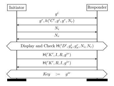
Figure 2: Bluetooth's Simple Secure Pairing Handshake
