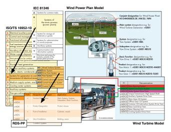
Fig. 2: Designation models IEC 81346, ISO/TS 16952-10, and RDS-PP and example energy information model for an energy plant [17].
