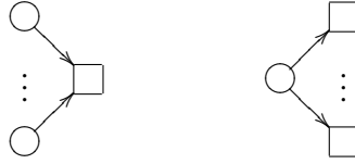
Figure 3.5: Free-choice nets: the two subnets from which any free-choice system can be built.
