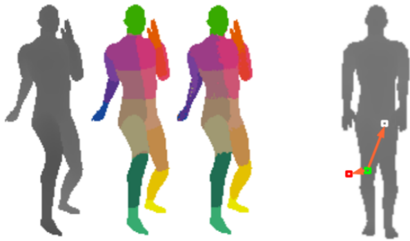
Figure 4. Left: Depth, ground truth body parts and predicted body parts. Right: A candidate feature specified by two offsets.
