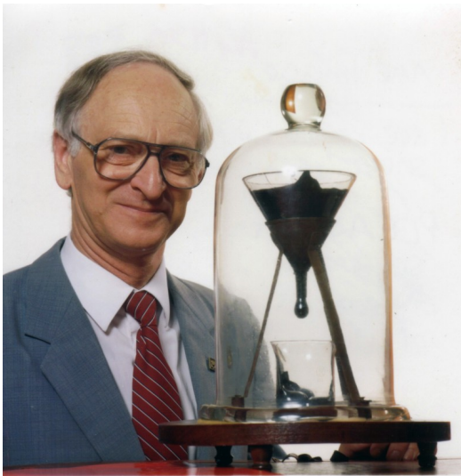
Pitchdrop experiment, Queensland. Experiment begun 1927 (1930). Drops fell in: 1938, 1947, 1954, 1962, 1970, 1979, 1988, 2000
