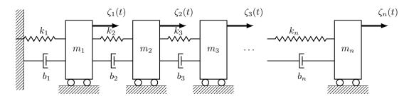
**Figure 1** *n*-body mass-spring-damper system.
