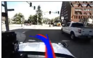
Fig. 1: Illustration of a motivating example where a vehicle is in front of an intersection. The sampled predicted trajectories using our approach are plotted in blue, where the ground truth future trajectory is plotted in red. In parallel autonomy, the autonomous system can leverage the predicted driver trajectory to avert risk and improve the driving. This requires the system to be confident of its predicted trajectories.
