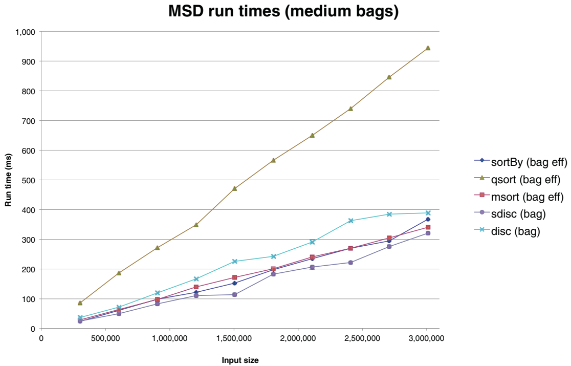
Fig. 18. (Colour online) Discriminator execution times for keys made up of medium-sized bags of small integers.
