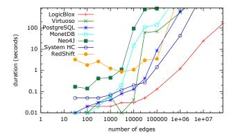
Figure 5: Running time of the 3-clique query on (increasingly larger subsets of) the LiveJournal graph dataset [26] using LogicBlox 4.1.4, Virtuoso 7, PostgreSQL 9.3.4, Neo4j 2.1.5, MonetDB 1.7 (Jan2014-SP3), a commercial in-memory column store (System HC), and RedShift. See [32] for full details and more experiments.
