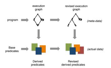
Figure 6: While the engine proper deals with maintenance of the derived predicates (materialized views) for a given program (left half), the meta-engine maintains the program under code updates and informs the engine proper which derived predicates should be revised (right half).
