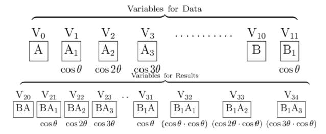
The variable belonging to each coefficient is written below it, as we have done in the diagram, by way of memorandum. The only further reduction which is at first apparently possible in the preceding result, would be the addition of  $V_{21}$  to  $V_{31}$  (in which case  $B_1A$  should be effaced from  $V_{31}$ ). The whole operations from the beginning would then be—
