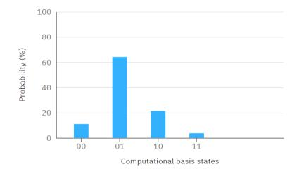
Qubits are prepared in a standard |0> state at the start of the computation.  Gates are applied to the qubits one after the other, as specified by the circuit. 3. Qubits are measured,yielding a bitstring (0 or1 for each qubit), aka a"measurement outcome"
