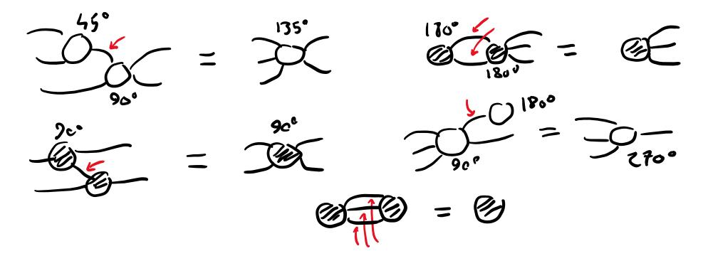
NB: Number of input/output legs is the same on both sides of the equation
