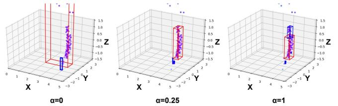
Figure 7: Clustering results with different  $\alpha$ . A small  $\alpha$  leads to loose clusters containing many noisy points. A large  $\alpha$  splits a human object into two clusters. Setting  $\alpha = 0.25$  gives the best empirical performance, as shown in the middle one.
