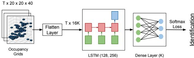
Figure 4: Classification Network Structure (see Sec. III-C).  $T$  represents the number of data frames used for identification and  $K$  represents the number of people to distinguish. Numbers in bracket represent layer sizes.
