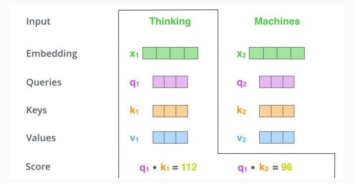
Then we rescale dividing by sqrt(Q) and apply softmax. O is the number of dimensions of the query  $[\mathbf{q}^{(t)}]_{0}$  and the  $\text{key } [\mathbf{k}^{(\tau)}]_{\Omega} \text{ (both }$ vectors need to have the same size to allow for the dot product)
