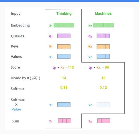
Computationally, we do all these calculations in parallel by using matrices rather than vectors. A matrix represents all the time steps in one go:
