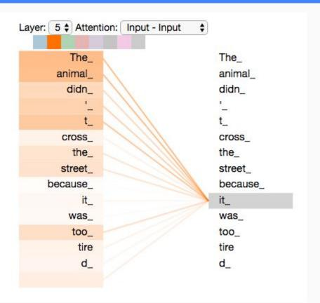
The attention mechanism is multiplicative. We first create a query, a key and a value vector per time step by linearly transforming each embedding:
