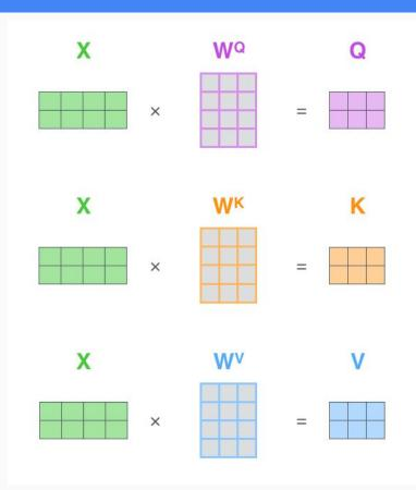
Computationally, we do all these calculations in parallel by using matrices rather than vectors. A matrix represents all the time steps in one go:
