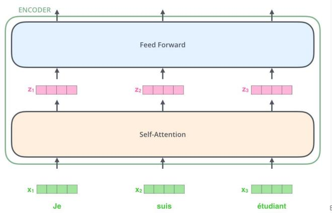
The new presentation per word  $[\mathbf{z}^{(t)}]_7$  that emerges from the self-attention layer, is then transformed with a feed forward fully connected NN into  $[\mathbf{r}^{(t)}]_{R}$ .
