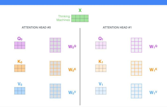
Another novelty of the transformer, is that it uses several attention channels in parallel. They are called 'heads', and their results are  $[Z^1]_{T7}$ ,  $[Z^2]_{T7}$ ,  $[Z^3]_{T7}$ , ...,  $[Z^H]_{T7}$  (H = number of heads):
