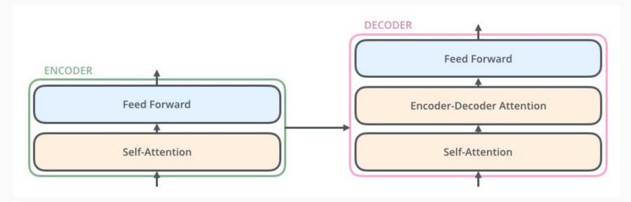
The first encoder receives an embedding  $[\mathbf{x}^{(t)}]_{x}$  per word (X = num)embedding dimensions). The self-attention layer mixes information across words, producing a new presentation per word  $[\mathbf{z}^{(t)}]_{7}$ , like the attention mechanism of a seq2seq.
