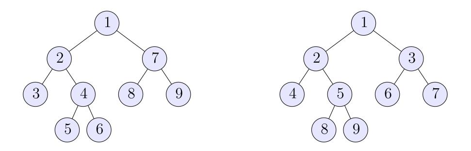
DFS (left) and BFS (right) on a tree, starting at vertex 1. The labels indicate the order by which the vertices are discovered.
