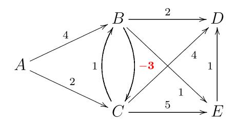
$\langle B, C, B \rangle$  is a negative-weight cycle: w(B, C) + w(C, B) = -2. There is *no shortest path* from source A in this graph!
