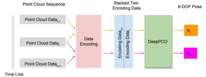
Fig. 1: System overview of the proposed DeepPCO framework. A sequential point cloud data stream is sent to the system. Two consecutive point cloud data are sent in parallel to the data encoding module, which implements the 2-D panoramic projection method. Projected depth images are then stacked to feed to DeepPCO neural network for predicting 6-DOF pose. These relative transformations are further combined to form a moving trajectory.
