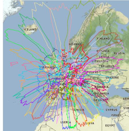
Figure 3: Footprint of a single randomly chosen Iridium satellite, comprising 48 antennas and their respective spot beams.
