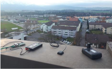
Figure 18: Picture of the measurement setup: Raspberry Pi 4, HackRF One, Iridium antenna, Iridium GO!
