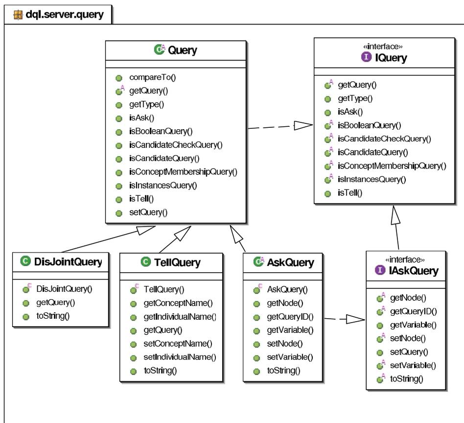
Figure 4.6: The UML class diagram of the query classes.
