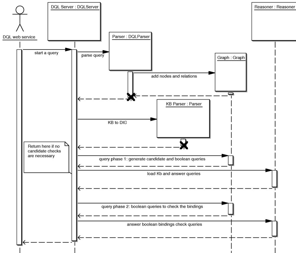
Figure 4.9: The UML sequence diagram for query answering.
