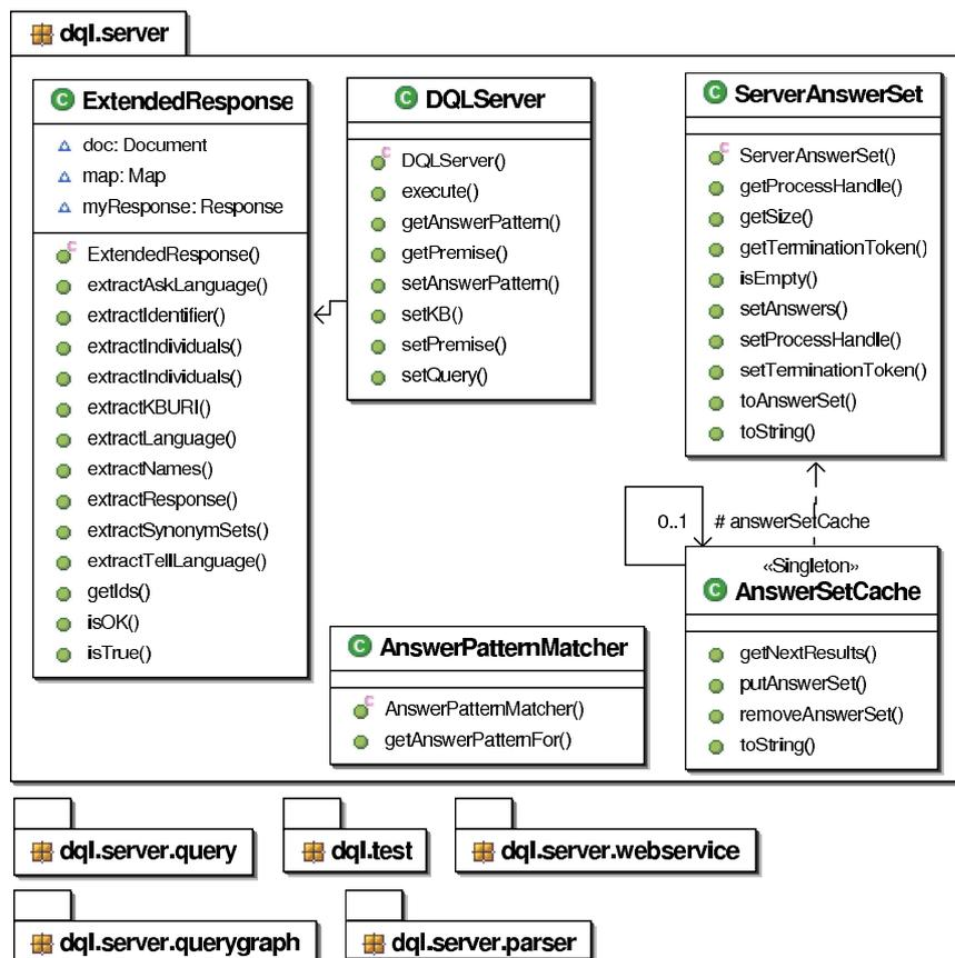
Figure 4.8: The UML class diagram of the package `dql.server`.
