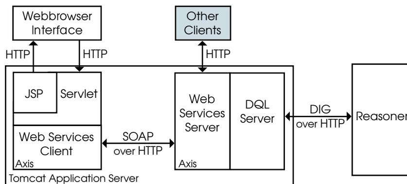
Figure 4.1: The chosen software architecture.
