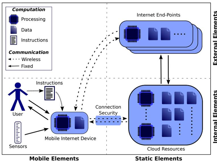
Fig. 1. Overall context showing internal and external elements in a mobile cloud computing system.
