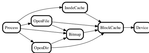
**Fig. 1.** Process network for MINIX file system
