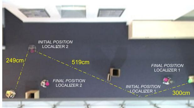
(b) Experimental setup with 2 localizers, clutter topology 2, localizer step-size is 50cm. The actual distances are marked. The faded Create robot images represent the start positions.
