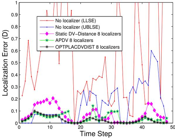
Fig. 8. Comparison of APDV with single-hop localization, Static DV-Distance and OPTPLACDVIDIST
