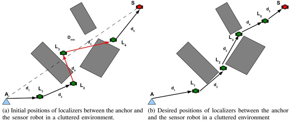
Fig. 2. APDV aims to align localizers between the sensor robot and the anchor node.
