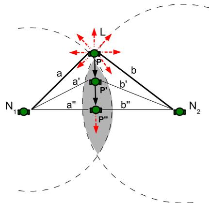
Fig. 4. Alignment procedure of  $L$  with neighbours  $N_1$  and  $N_2$ .  $L$  chooses the direction (out of  $N_{dir}(=8)$  directions) which offers the maximum decrease in the sum of distances to its neighbours ( $a+b$ ). The procedure completes when condition  $(a' + b') < (a + b)$  no longer holds.
