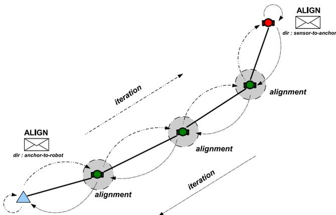
Fig. 3. Working of the APDV algorithm towards refining the distance measurements obtained via initially through the shortest-path-distance search of the DV-Distance algorithm.
