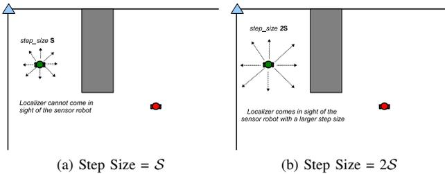
Fig. 5. Step Size Threshold in APDV algorithm
